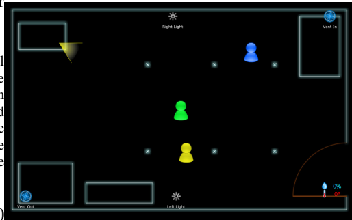
Fig. 3. Example view of a Domatiq panel application. Locations: left top edge - a single PrimeSense sensor; top right and left bottom vents operator points; in the middle of the top and bottom light operator points. There are also visible three users in different states: (from top) the tracked user, the user in a command mode, and the user who selected an operator point.
